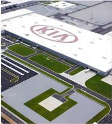
KIA Motors Mtg. Facility (One of Largest Industrial Roof with preformed TPO Membrane w/p project)
