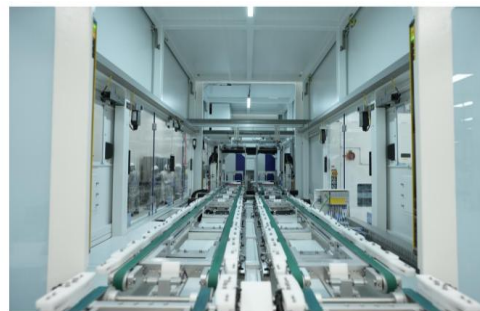
Automated Wafer Transfer System Inside Cell Factory
