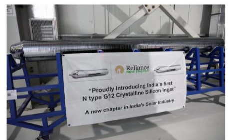
First Ingot (300 mm diameter and 2.85 m length)
