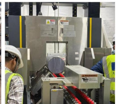
Machine for Slicing Ingot into Wafers
