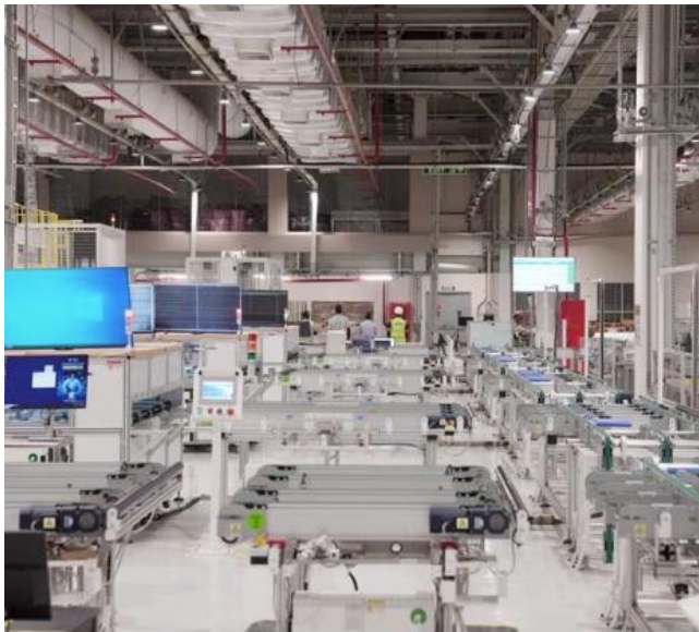
Pre-lamination Testing Station [including Electroluminescence (EL)]
